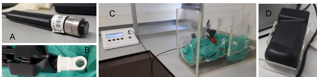
Figure 2.14 - Biometry equipment. A - Probe of the Corneometer ® ; B - Probe of the Tewameter ® ; C - Tewameter ® ; D - Camera of the Visioscan.
