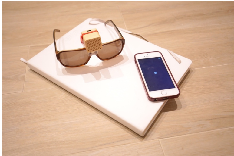
Figure 22: Sonar Glasses version 1. A bluetooth speaker poorly attached on a sunglass.
