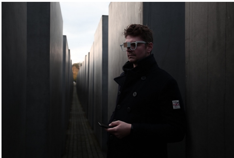
Figure 25: A young man interacting with solid squared pillars using the Sonar Glass. Listening obstacles through echoes produced by a digital sound source fixed on forehead. Memorial to the Murdered Jews of Europe, Berlin, Germany, 2020.
