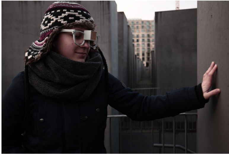
Figure 24: A young woman interacting with solid squared pillars using the Sonar Glasses. Listening obstacles through echoes produced by a digital sound source fixed on forehead. Memorial to the Murdered Jews of Europe, Berlin, Germany, 2020.
