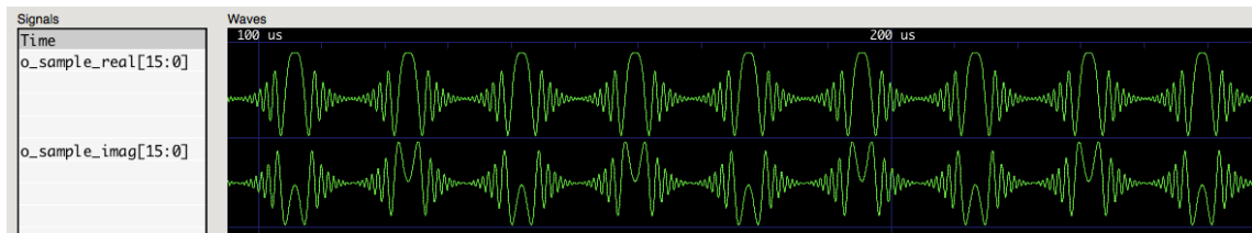
Figure 5.11: Interpolation waveforms generated from circuit simulation.
