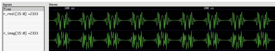
Figure 5.13: Decimation waveforms generated from circuit simulation.
