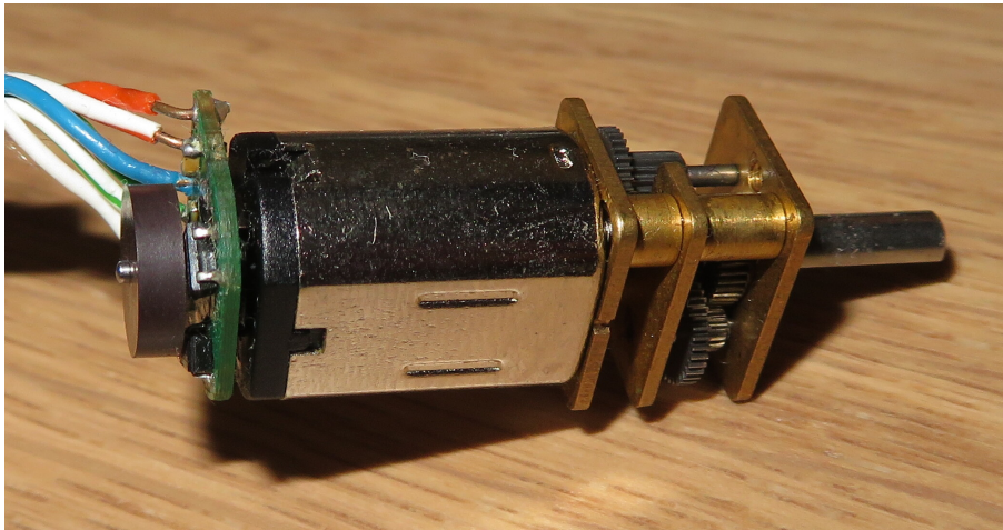
Figure 4.2: Detail of the DC gearmotor and attached magnetic encoder
