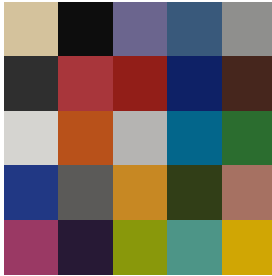
Figure 3.15: Image with 100 \times 100 resolution, to be corrected, where the top-left 20 \times 20 square is filled with the sample color to be corrected and the remaining 24 with the color chart patches.
