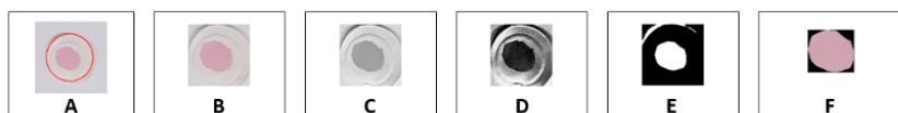
Figure 2.7: Color extraction steps. A: Hough transform applied for disk detection. B: Cropped Disk. C: Grayscale B. D: Result of C normalisation and histogram equalisation. E: Binarisation of D. F: Sample after detection. [4]
