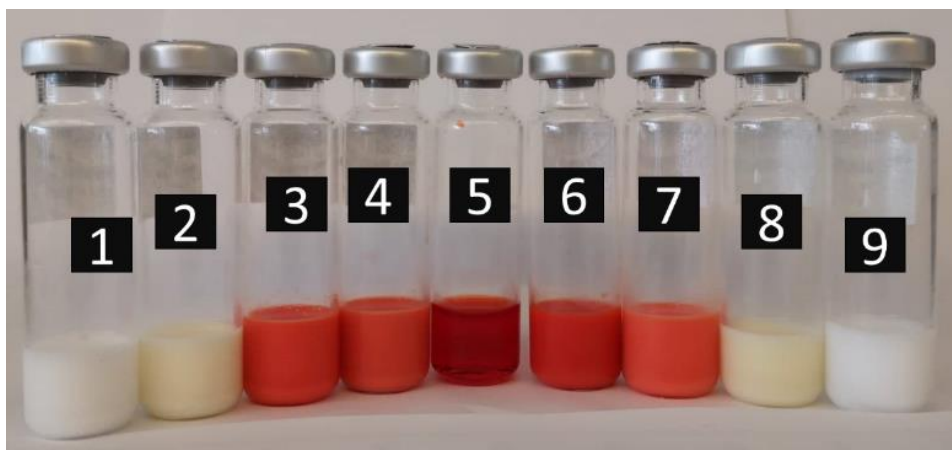
Fig. 4.2: NLCs with different compositions and Dox-free. 1) NLC_{(Pal)} , 2) NLC_{(Pal-PEG-FA)} , 3) NLC_{(Pal-DOX)} , 4) NLC_{(Pal-DOX-PEG-FA)} , 5) DOX_{(free)} , 6) NLC_{(Gel-DOX-PEG-FA)} , 7) NLC_{(Gel-DOX)} , 8) NLC_{(Gel-PEG-FA)} , 9) NLC_{(Gel)} .
