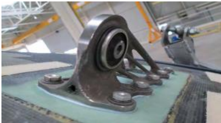
Figure 21 - Airbus ALM/3D Printing FCRC Cabin Bracket Installation[69]
