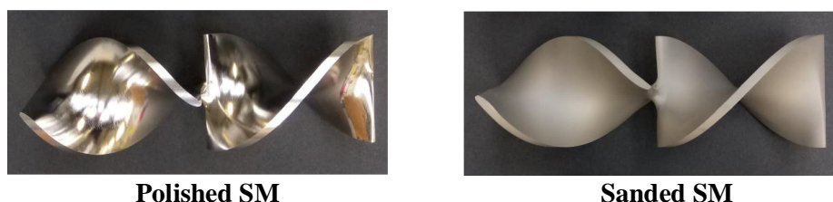
Figure 2.1 – Kenics ® SM as obtained (polished SM) and after sanded treatment (sanded SM).
