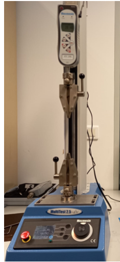
Figure 3.21 Machine set up to uniaxial tensile tests.
