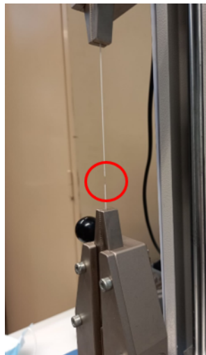
Figure 4.10 PCL printed filament response to uniaxial tensile test.
