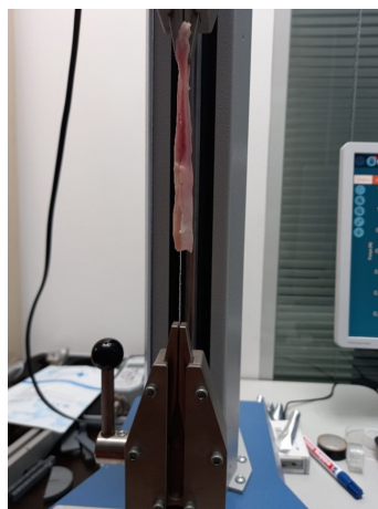
Figure 3.22 Ex vivo uniaxial tensile testing set up.
