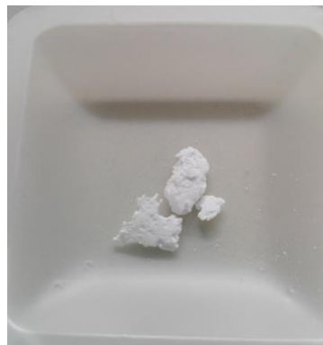
Figure 4.1 - Neat PLLA microparticle's agglomerates after production.
