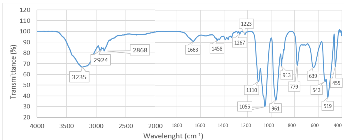
Figure 4.16 - FTIR spectra of the synthesized chitosan/GPTMS/ \beta -GP hydrogel without PLLA microparticles.
