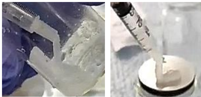
Figure 4.3 - Preliminary injectability of a 1.5% MPs sample through a syringe
