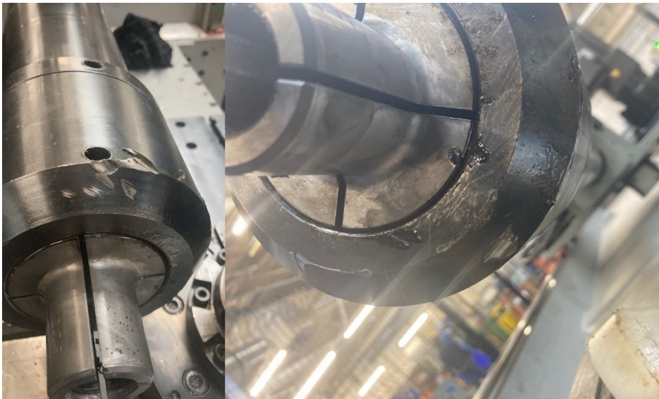
Figure 3.2: Carriage damage due to manual collision in 9611 e-MOB axis
