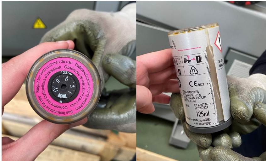
Figure 3.9: Lubrication unit from one of AMOB's machines from two perspectives
