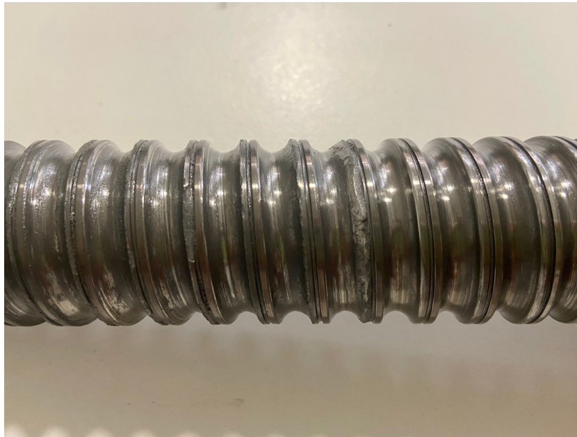
Figure 3.10: Replaced ball screw with severe wear signs
