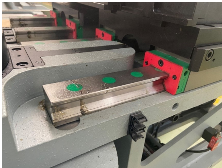
Figure 3.5: Linear guide in one of AMOB's machines
