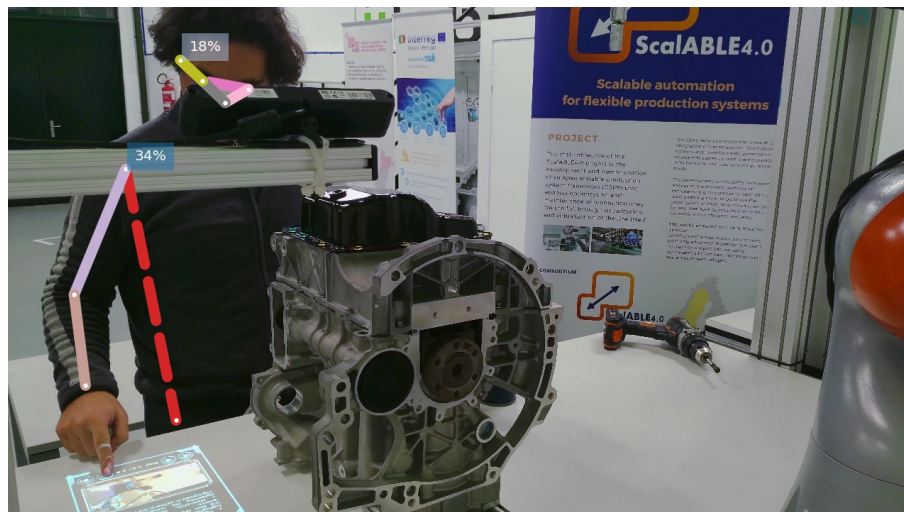
Figure 4.11: Example of rendered frame where OpenPifPaf did not fully associate detected joints as part of the same skeleton.
