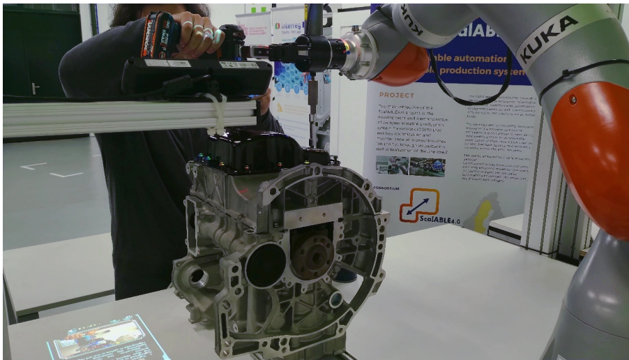
Figure 4.13: Example of rendered frame where OpenPifPaf did not detect the visible operator.
