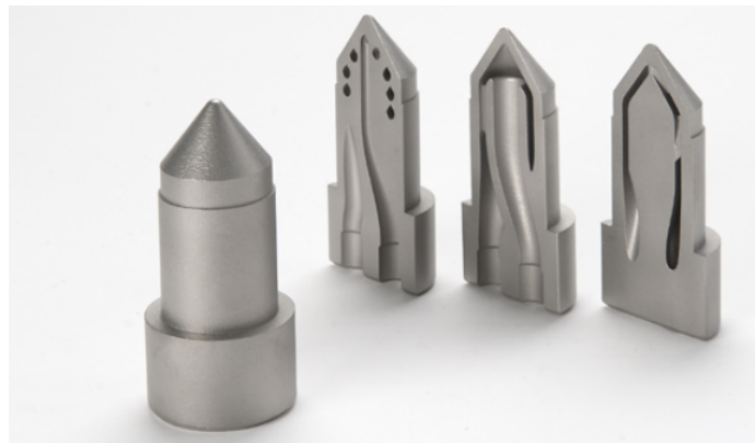
Figure 2.22 Tooling insert equipped with conformal cooling channels [32].
