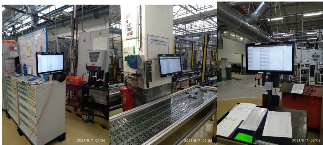
Figure 31: Tablets positioned in the end of the production lines in the WPS
