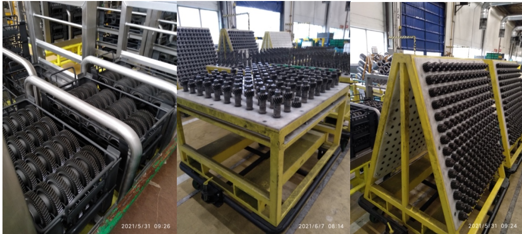
Figure 15: Pieces after the dust blasting process
