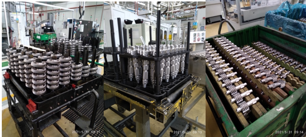
Figure 13: Pieces ready to receive thermic treatment
