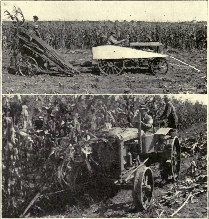
FIG. 7.—IMPROVED DEVICE FOR PICKING UP LODGED CORNSTALKS
