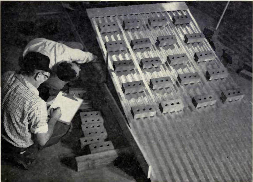
Aluminum roof section loaded both sides; 12-foot span. Test 2.
