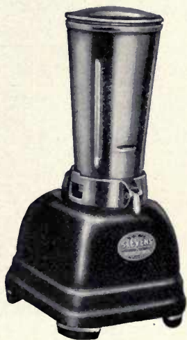
Fig. 8.—The paper plaques were reduced to pulp in this machine in order that the bacteria enmeshed in the fibers could be counted.
