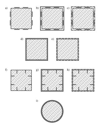
**Fig 1.** Proposed strengthening solutions for structural elements in compression using CFRP materials
