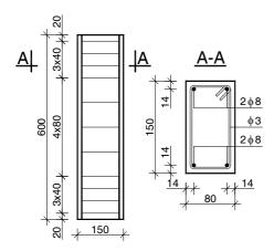
Fig 2. RC columns tested. Elements S1a and S1b
