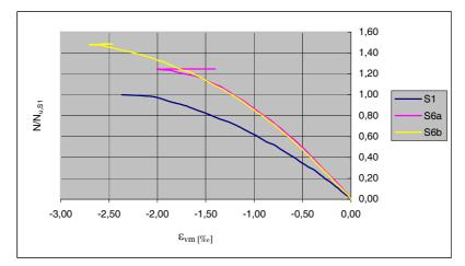
Fig 6. N/N $_{u,S1}$  versus  $\epsilon_{vm}$  for columns: S1, S6a, S6b
