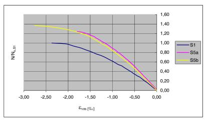
Fig 5. N/N $_{u,S1}$  versus  $\epsilon_{vm}$  for columns: S1, S5a, S5b
