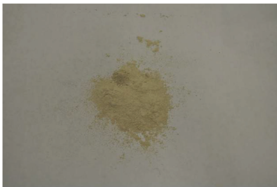
Extracted concrete powder sample
