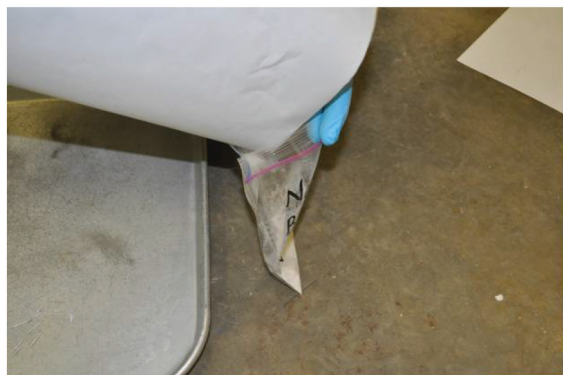
Transfer of concrete powder to plastic bag
