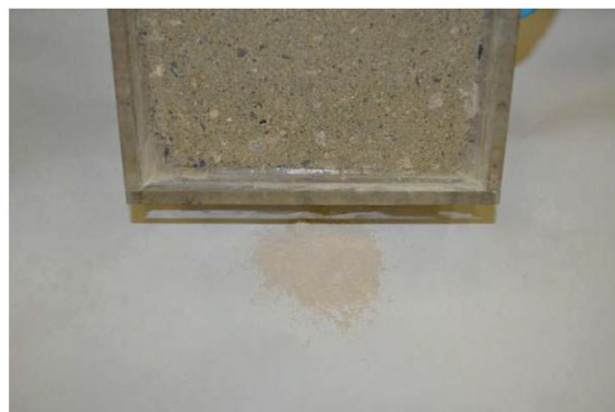
Extraction of concrete powder
