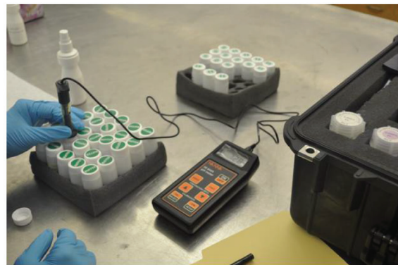
Testing of total water-soluble chloride content of concrete by RCTW method
