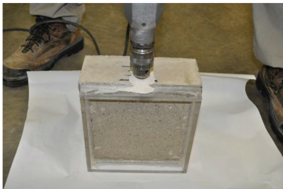
Drilling into concrete prism
