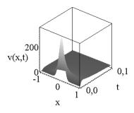
Figure 2. The final velocity distribution of  $v_1 = \frac{1}{t^{\frac{1}{2}}}g\left(\frac{x}{t^{\frac{1}{2}}}\right)$  for the paramter set of  $c_4 = 0.2, a = 0.27, \nu = 40, \rho_1 = 2, \rho_2 = 20.$
