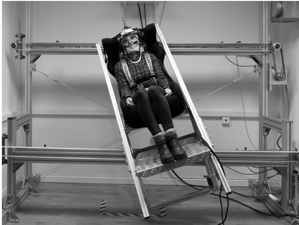
Figure 12. The mechanized sled used for whole-body manipulation during vestibular stimulations. The head is stabilized using an extriction collar and hook-and-loop straps. The chair rotates on two belts powered by dedicated servo motors, while the eye movement responses are monitored using the head mounted Chronos Eye Tracker worn by the subject. Reprinted from Wibble T, Pansell T. Vestibular eye movements are heavily impacted by visual motion and are sensitive to changes in visual intensities. Invest Ophthalmol Vis Sci. 2019;60:1021–1027. © 2019 The Authors. Published by the Association for Research in Vision and Ophthalmology (ARVO).
