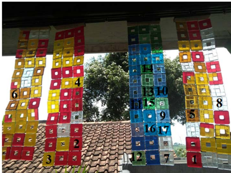
Figure 4 The luminance measurement points over the glass curtain surface.
