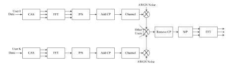
Figure 1 Baseband signal model of uplink OFDMA system.
