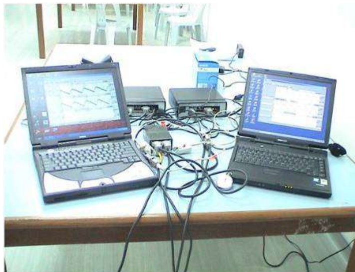
Figure 1 Apparatus for two-channel PPG recording using two independent systems.
