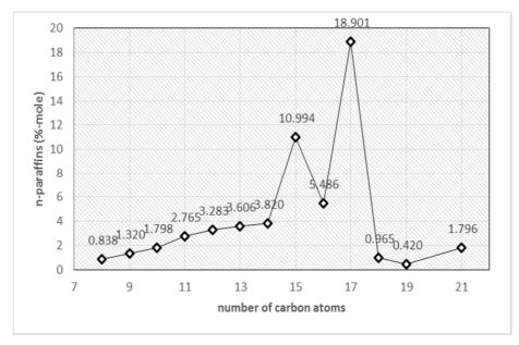
Figure 4 Formation of paraffins during decarboxylation of Mg-Zn basic soap.
