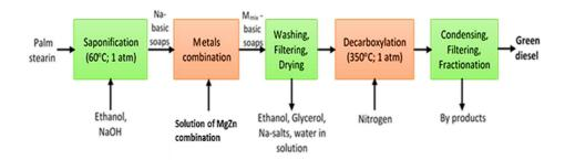
Figure 1 Flowchart diagram of soap-derived green diesel production.
