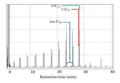
Figure 2 GC-FID chromatogram patterns for liquid bio-hydrocarbon fractions.
