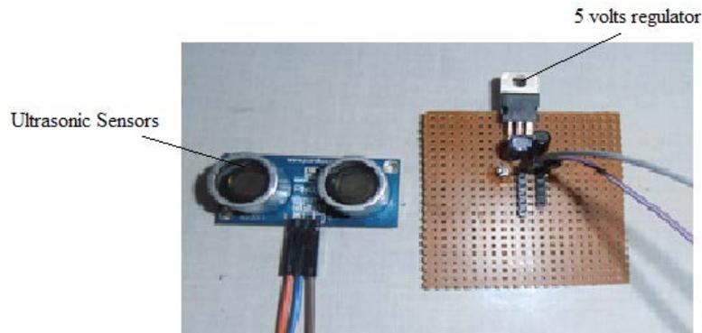
**Figure 4** Ultrasonic sensor connected to 5V regulator.
