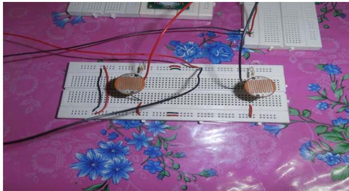
**Figure 10** Circuit design of the light detection sensors.
