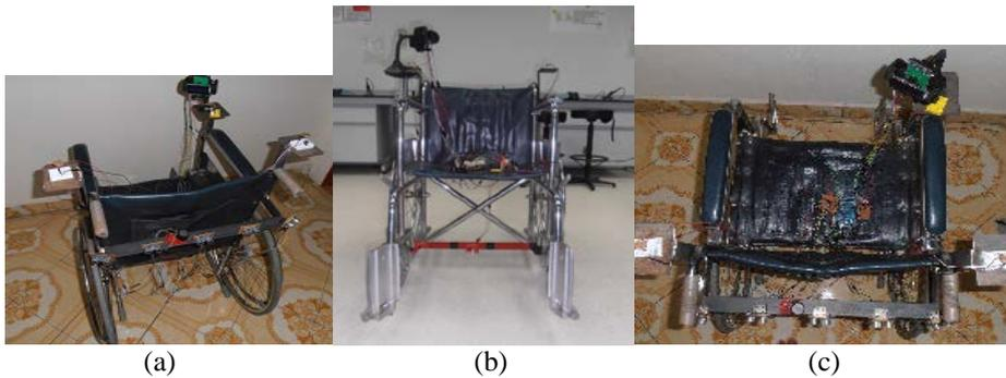
**Figure 17** (a) Back view (b) front view, (c) top view of proposed wheelchair kit.
