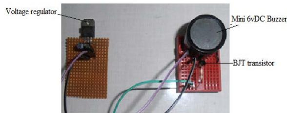
**Figure 5** Emergency alarm system connected to 6-volt regulator.
