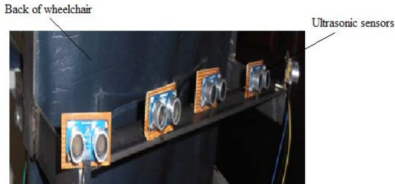
**Figure 14** Installation of 5 ultrasonic sensors.
