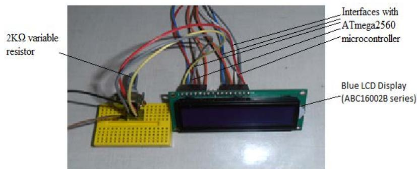
**Figure 3** Blue LCD display set up.
