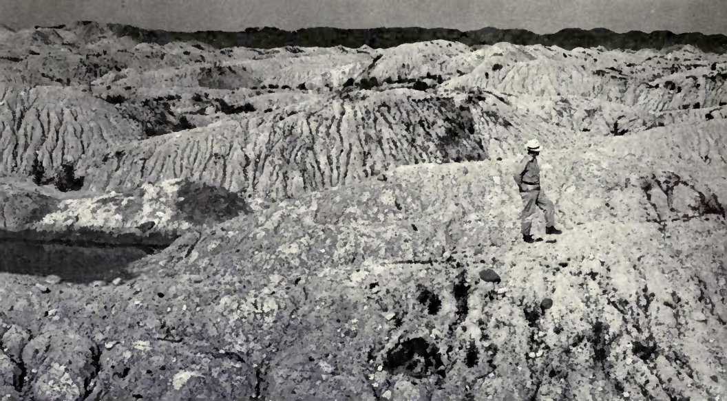
Calcareous, sandy, silty clay spoils like these, with cemented surfaces, predominate in Will and Grundy counties. Of the nontoxic spoils in the state, these are the most difficult to reclaim. Natural vegetation is very sparse for many years after stripping. (Fig. 8)
