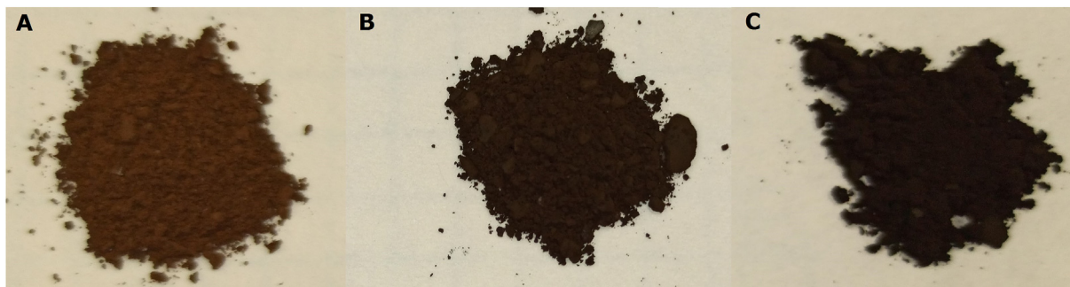
Fig. 3. Photographs of the HTT biochars obtained at different processing temperatures (A) 200 °C (B) 275 °C (C) 300 °C.
