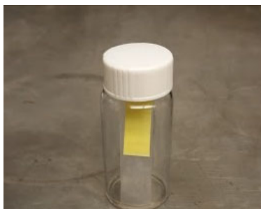
Figure 2.2 Set up for amygdalin (0-100 \mu\text{g} \text{CN}^- equivalent) + 50 \mu\text{L} of 3 U/mL \beta -glucosidase enzymes in pH 8 phosphate buffer and the picrate paper test strip.
