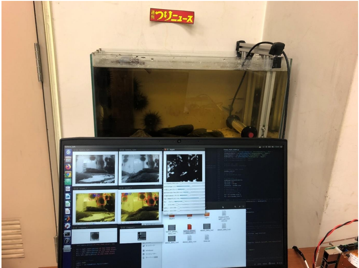
Fig. 5-35: Experimental run diagram of the sea urchin recognition system using underwater stereo vision.
