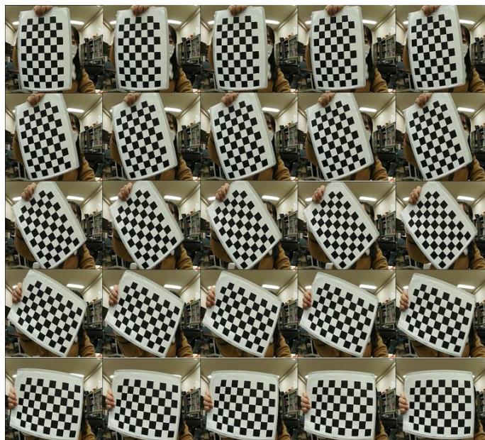
Fig. 2-7: Binocular camera calibration images.
