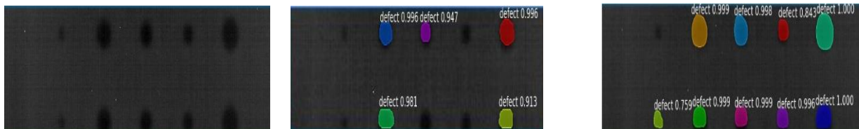
(c) Example 3 from plexiglass specimen (left: ground truth; middle: training without synthetic data; right: training with synthetic data)
