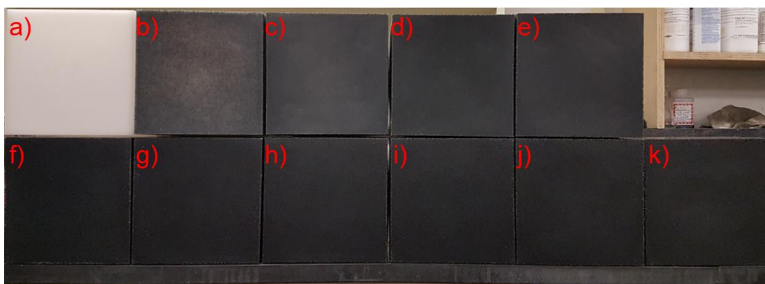
Figure 13. Pictures of the rotomolded parts with different GTR contents: (a) 0, (b) 5, (c) 10, (d) 15, (e) 20, (f) 25, (g) 30, (h) 35, (i) 40, (j) 45 and (k) 50 wt.%.
