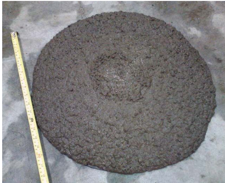
Figure 4.10: Typical consistency of the 0.45 w/b ratio mixture showing a VSI of 0
