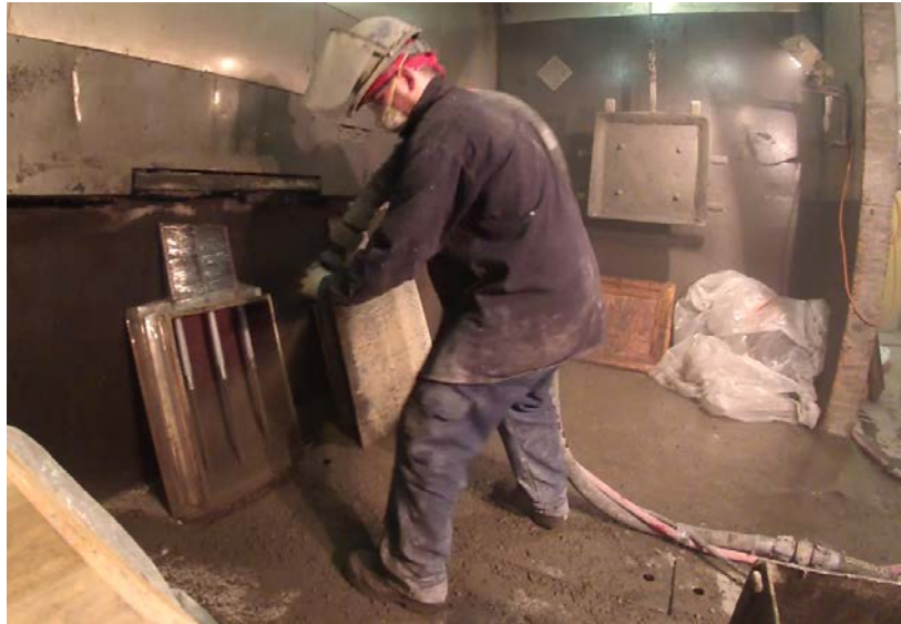
Figure 2.3: Molds containing the “pull-out” specimens
