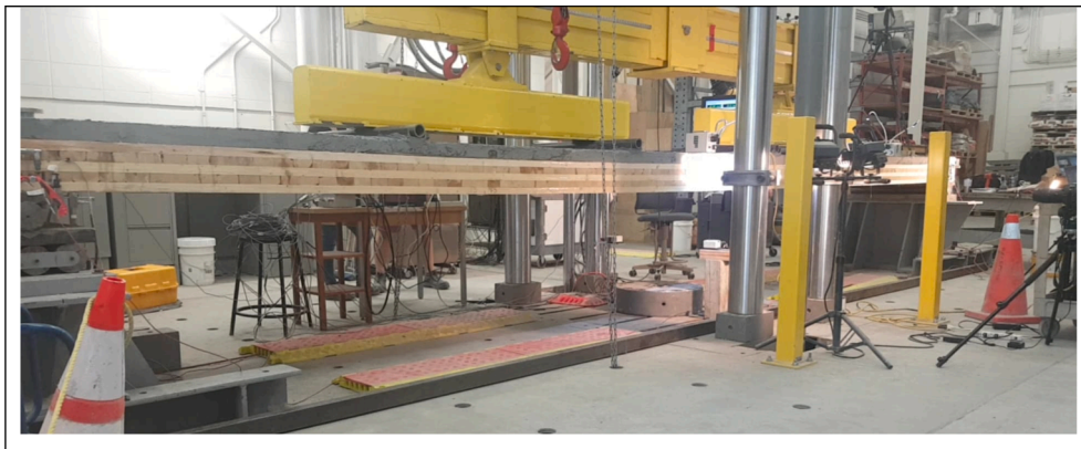
Fig. 6. Photo of a bending test on a CLT-HPC floor in the laboratory.
