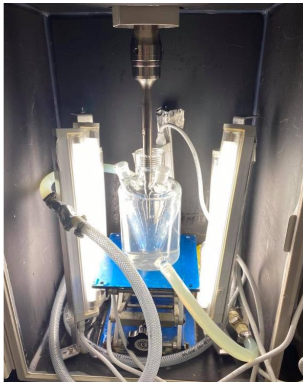
Figure 6-4 Illustration of the sonophotocatalysis experimental setup.
