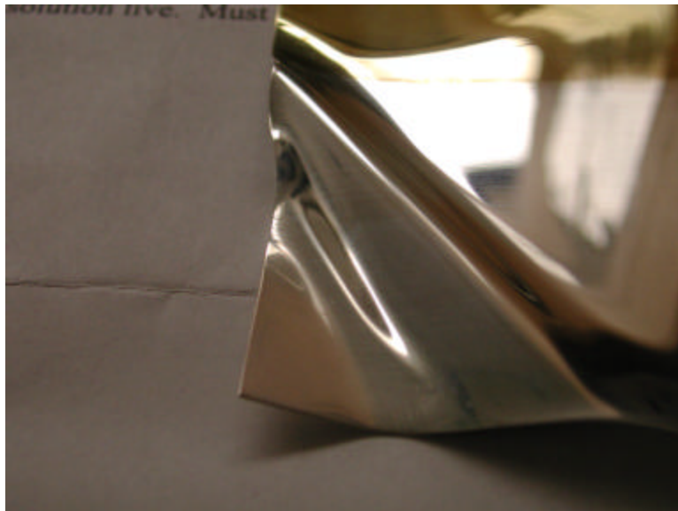
Figure 11 Adhesion test (pass) of bright silver over polished brass. Solution from Supplier No. 2
