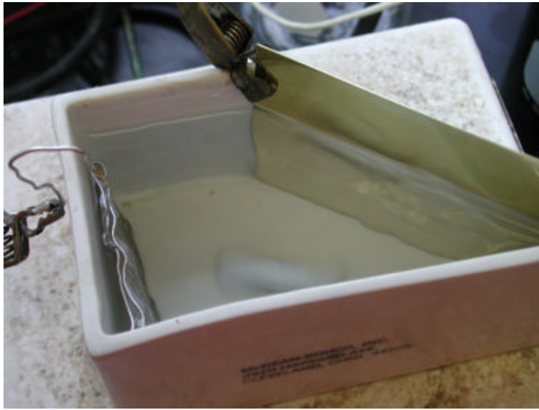
Figure 3 Hull Cell Apparatus, Brass panel being plated with non-cyanide silver from supplier No. 2. agitation is via a magnetic stir bar, anode is made of solid platinum mesh.
