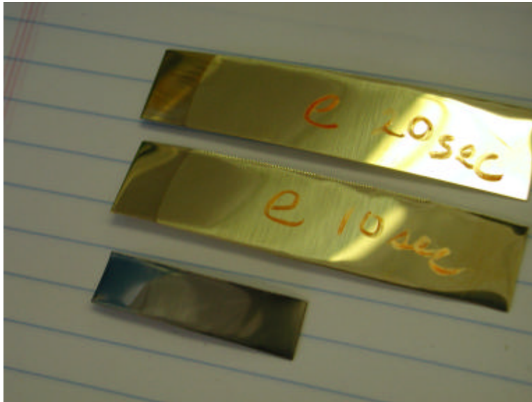
Figure 4 Immersion silver deposits on brass (upper two strips) and bright nickel after 10 and 20 seconds immersion in non-cyanide process from Supplier-1
