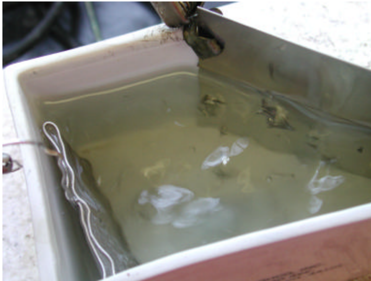
Figure 10 Adhesion failure during silver plating of non-cyanide silver over bright nickel. Silver solution from Supplier No. 1
