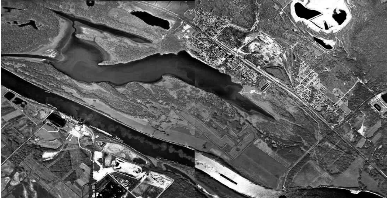
Figure 2. Composite of two 1994 infrared aerial photographs of Lake DePue (USGS, 1999). Note the white sediment plume from the South Ditch entering the northeast end of the lake. USGS Upper Midwest Environmental Science Center, Kewaunee, Wisconsin, images 161-011-pe-1994i and 161-009-pe-1994, 1:24,000.
