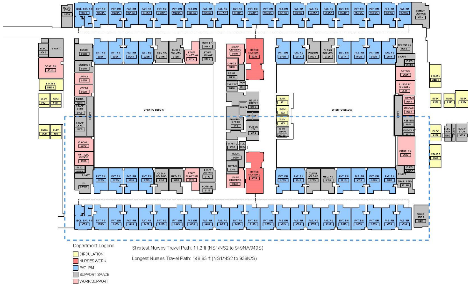
Figure 1. Floor plan of the 9 South in the Atrium building (Image Courtesy: RUMC, designed by Hansen Lind Meyer, plan re-drawn by the research team). Please see the dotted lines for area related to study and the drawing is not to scale.
