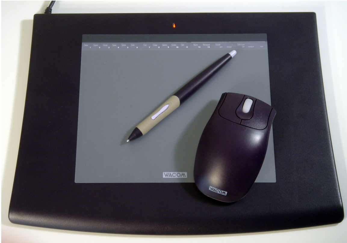
Figure 6.7. Photograph of the Wacom Intuos2 digitizing tablet used for testing and development of the present application. Although the mouse device is included with the tablet, its features were not used with the application.
