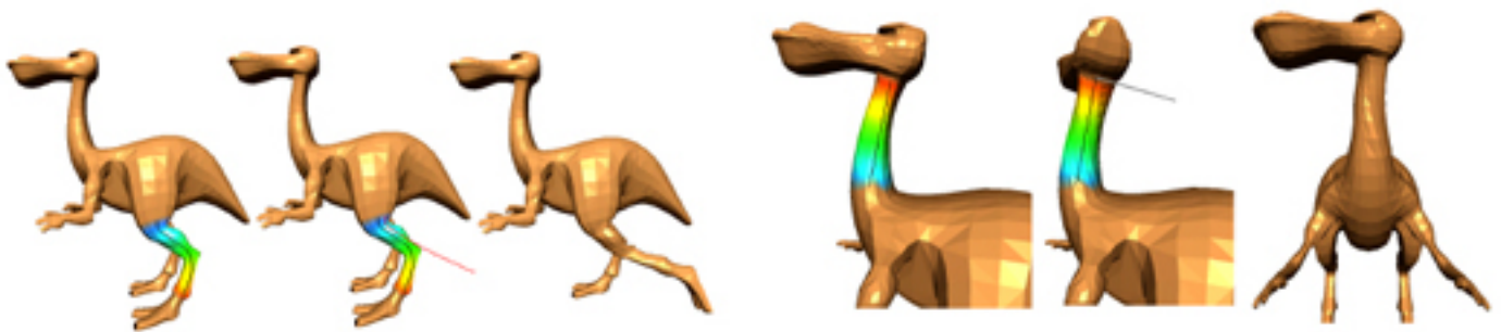
Figure 5.20. (left) The leg of a mesh model of a dinosaur is straightened to follow the path of a red deformation stroke. (right) The model's head and neck are turned to follow manipulations of a deformation of an orthogonal deformation stroke. [Kho & Garland, 2005]
