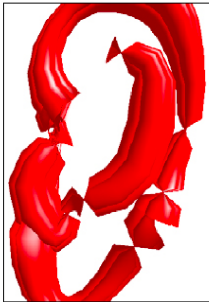
Figure 7.7. An example of the effects of Frenet frame twist from Davison's human ear modeling system [Davison, 2003].
