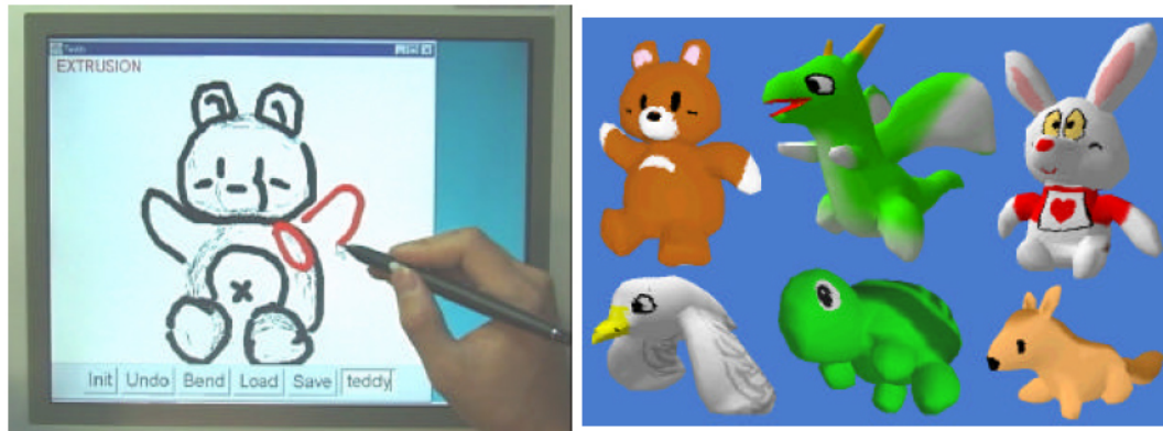
Figure 5.8. (left) A user creates a 3-D model of a teddy bear from silhouette strokes using Igarashi et al. 's Teddy modeling system [Igarashi et al. , 1999]. The system ‘inflates’ the user’s silhouette strokes to create a triangle mesh model. (right) Several example models from the system. These models have been colored with a commercial texture mapping software, however later versions of the Teddy system included the ability to color models directly within the program.
