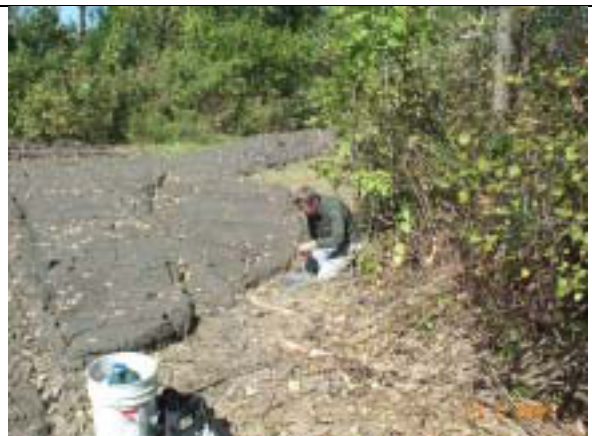
Fig. 24. Material placed at the Powers site maintained its shape, but could not support a person's weight on October 7.
