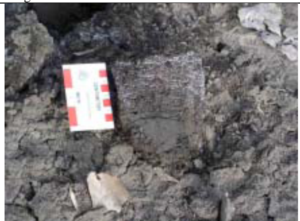
Fig. 26. Ice crystals laced the sediment for about three inches below the granular material. Below that the sediment was moist and plastic.
