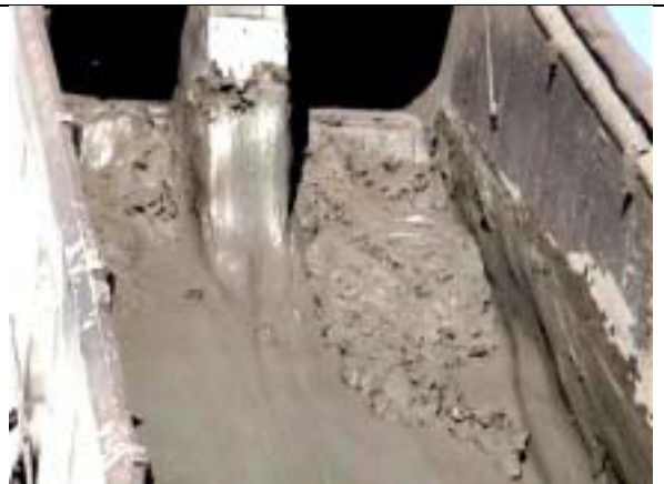
Fig. 18. Small amounts of sediment occasionally hung up in the corners of truck beds. This sometimes was associated with residue from a prior load of another material such as lime.
