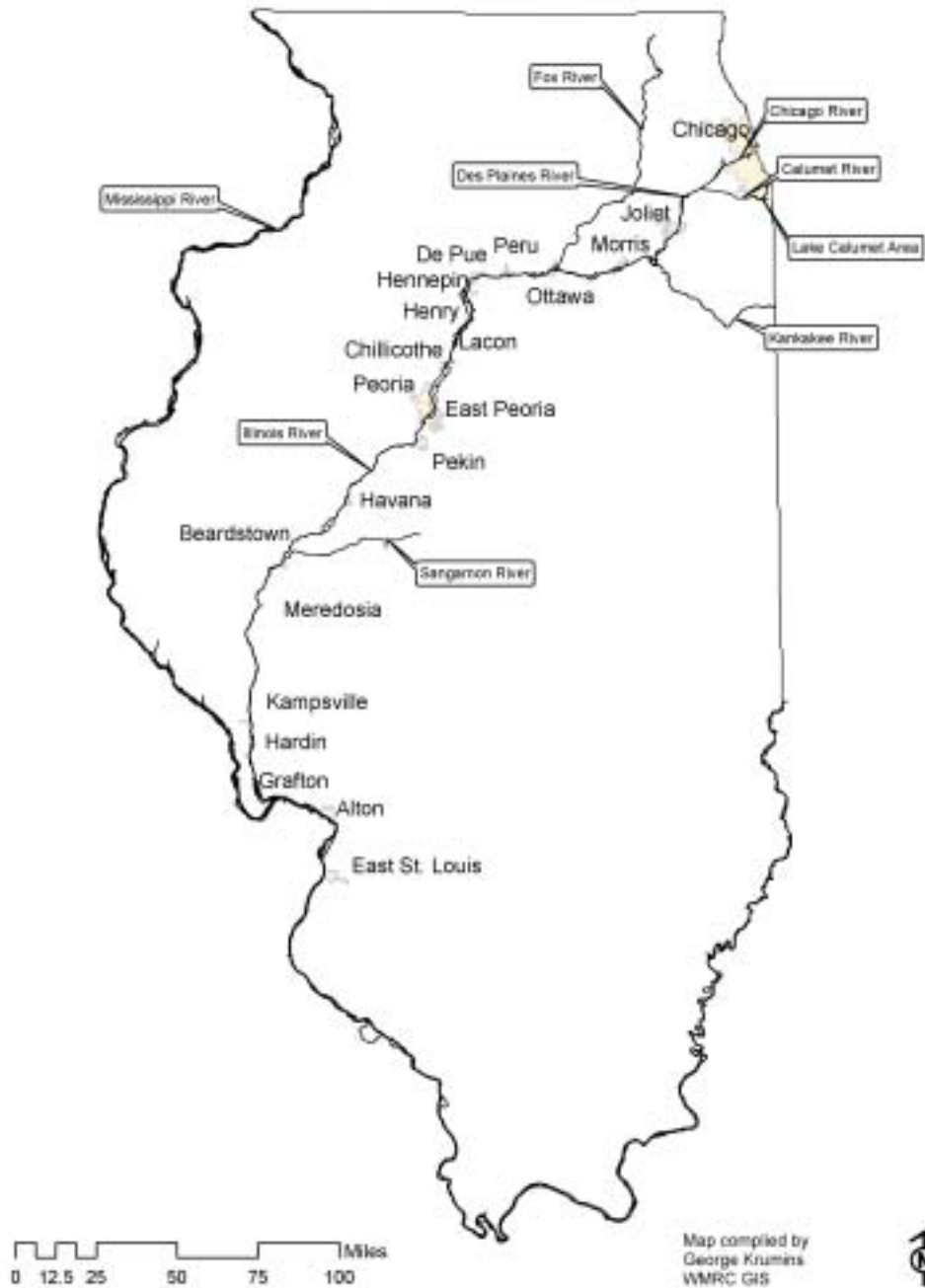
Fig. 1. Sediment for the transport demonstration was collected at East Peoria in shallow water near the daymark at river mile 165.3 where the Spindler Marina boat channel meets the navigation channel. It was then taken by barge to the Paxton 1 landfill site near Lake Calumet in Chicago. The Illinois Waterway connects the Mississippi River with Lake Michigan. The Illinois River proper extends from Grafton, northeast of St. Louis to mile 273 near Joliet. There it is formed by the confluence of the Kankakee and Des Plaines Rivers. The waterway follows the Des Plaines and then branches to Lake Michigan via the Chicago River to the north and the Calumet River to the south. The entire system is navigable by barges.
