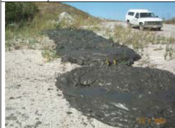
Fig. 23. Sediment stayed in place along the side of the roadway leading up the landfill flowed only a few inches downhill. The slope is 8%.
