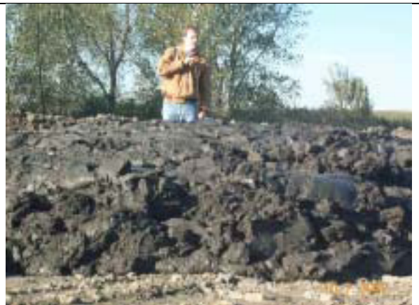
Fig. 20. Sediment retained its consistency despite handling.
