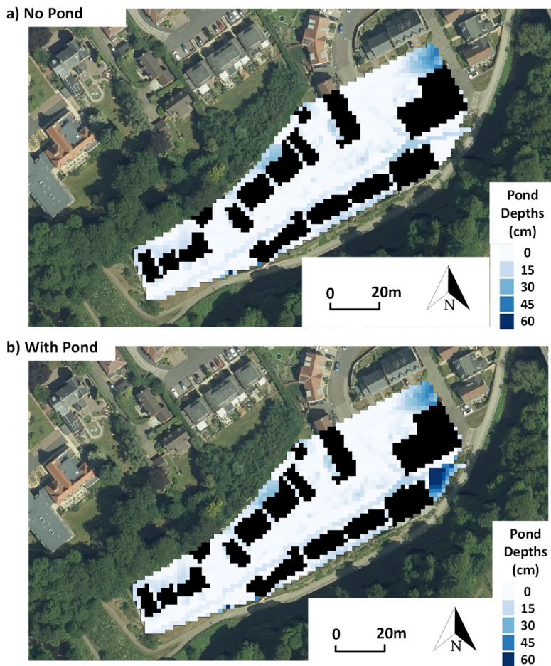
Figure 3: Simulated maximum water depths at Juniper Green for a 15-minute one-in-100-year event with dry initial conditions. (a) With no pond; and (b) With a pond. The buildings are shown in black.
