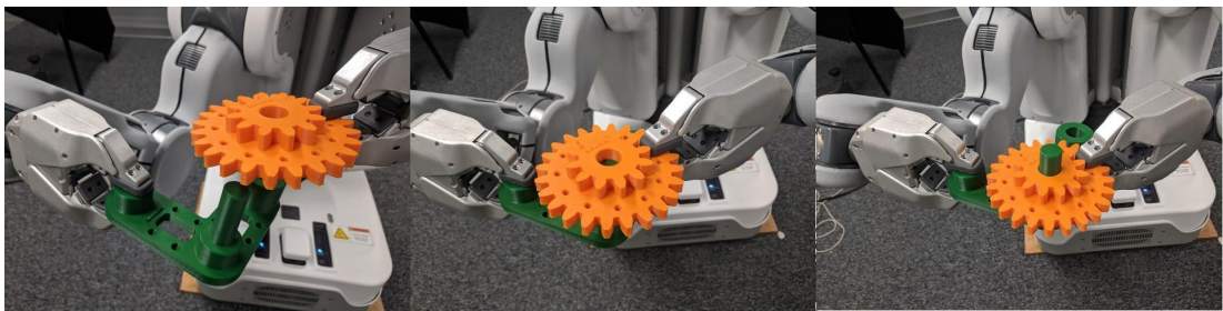
Figure 19: The execution of a neural network policy for inserting the gear on the peg.
