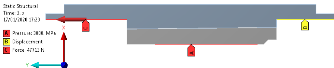
Figure 4.14: Structural conditions of the compound cylinder.
