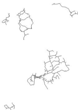
Figure 3.4: Three situations leading to a largely disconnected road network. Top: hamlet for which the access clearly lies outside the main area. Middle: a very small but critical road section is administratively in another LAD. Bottom: the whole area is formed of islands.
