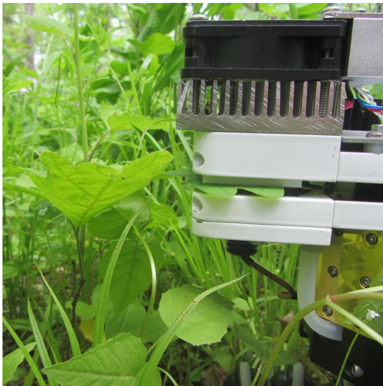
Figure 27. LI-6400 sensor head clamped onto a white oak seedling leaf in the oak savanna restoration study site at Nachusa Grasslands, IL, USA (Picture by S. R. McCarragher).
