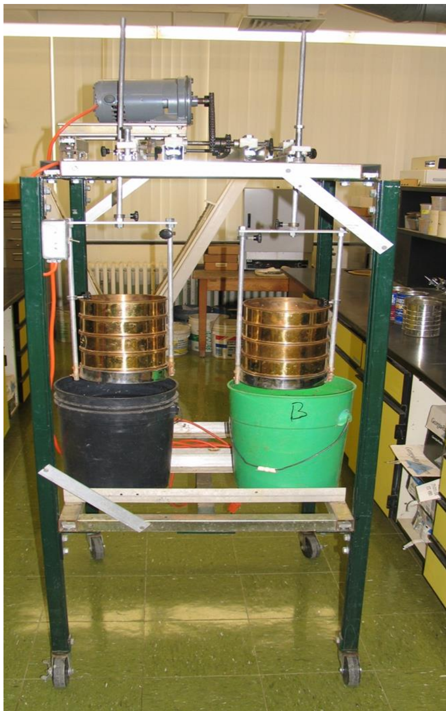
Figure 31. Image showing the motorized platform built by M. Wander and M. Konen (as per Kemper and Rosenau 1986), used to agitate the soil samples to measure wet aggregate stability (Picture by S. McCarragher).
