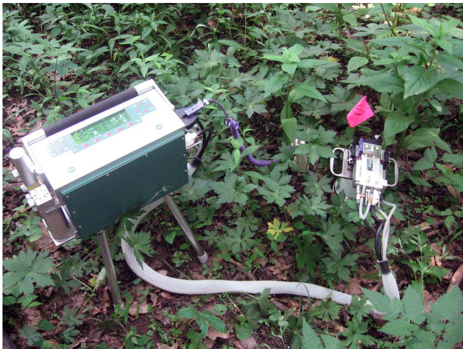
Figure 30. 6400-09 Soil CO 2 Flux Chamber attached to the sensor head of the LI-6400 with the attached soil temperature probe measuring soil temperature at approximately 15 cm below ground.
