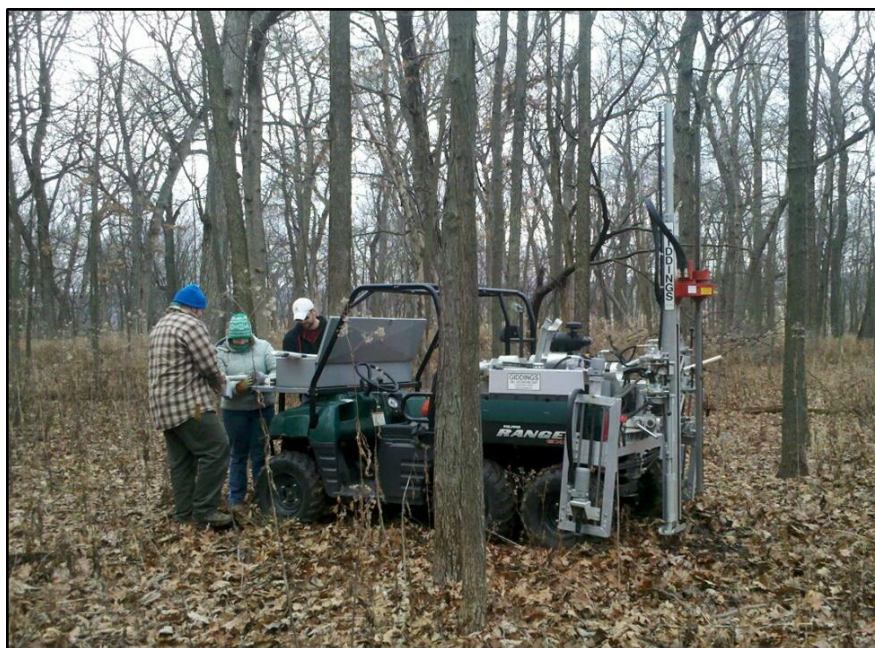
Figure 29. Image showing the trailer mounted Giddings HDGSRPT-#25 hydraulic soil coring machine (Giddings, Windsor, CO, USA) used to collect the 5 meter soil cores (n=40) in the eastern tract of the oak savanna restoration study site at Nachusa Grasslands, IL, USA (Picture by M. Konen).
