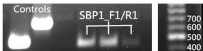
Figure 25: Electrophoresis of colony PCR of SBP1 in pSTARGATE vectors in Agrobacterium .
