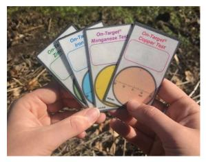
Figure 7.1 Selection of radial detection cards for zinc, iron, manganese, and copper from Access Sensor Technologies, LLC.
