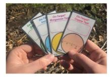
C. Radial distance-based detection cards for Zn, Fe, Mn, and Cu
