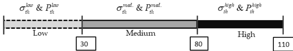
Figure 3.2. Scale for choosing the uncertainty threshold (the figure is not drawn to scale)
