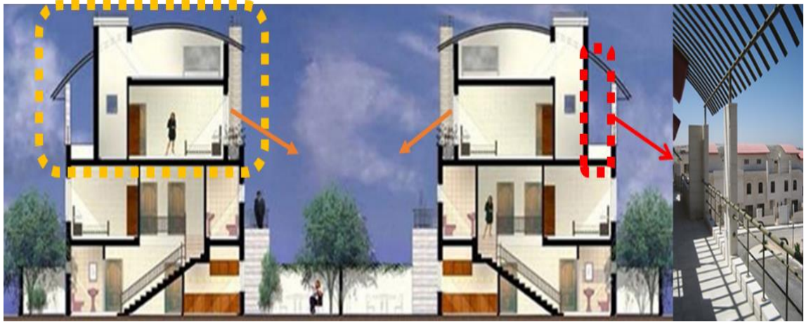
Figure 5.3 A cross-section in a terraced house from King Abdulla city. The upper deck (yellow square) forms a separate apartment from the lower deck house overlooking private gardens of these houses. The passage that links the upper deck apartments is a shared semi-public access, and residents cannot use it as an open private space
