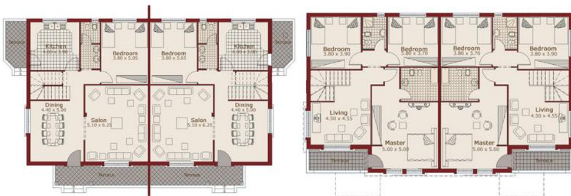
Figure 4.10 Floor plans of the “luxurious” built semi-detach houses in King Abdulla city (Mawared co)
