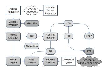
Fig. 2. Components of the *webinos* policy framework on a device. Requests come from either local or remote sources, and are then managed by the Decision Wrapper. Policies are held on a PZP and may depend on data fetched from the rest of the personal zone
